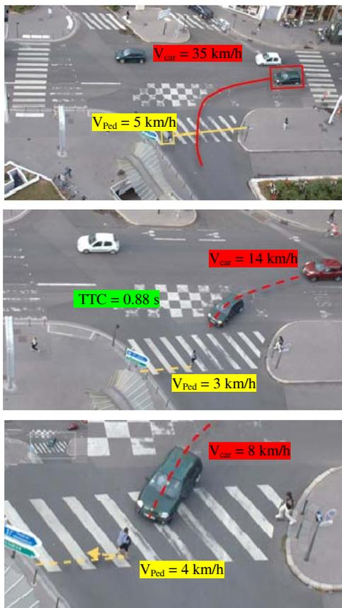
Full line = expected trajectory / Dotted line = real trajectory
